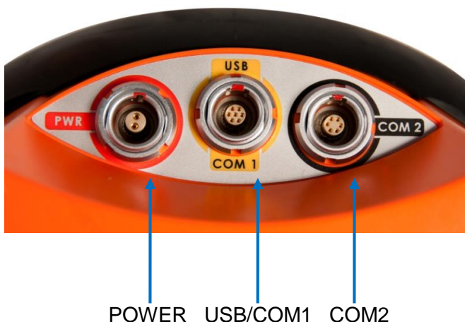
Figure 1: SF-3040 Connectors, Detail
