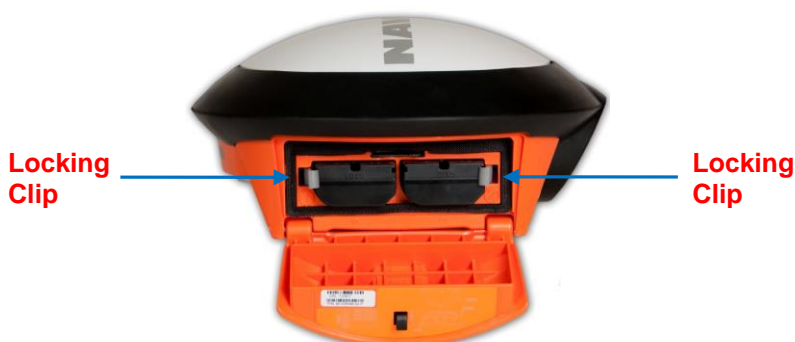
Figure 13: Battery Packs Installed in Chamber Showing Locking Clips
