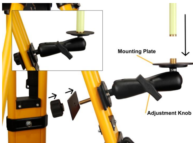
Figure 81: Mounting the Radio Antenna Bracket
