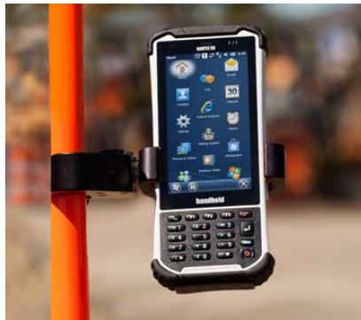
Figure 23: Mounting the MicroSurvey Nautiz X8
